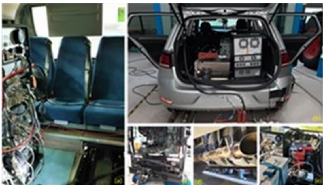
Figure 1. CRMT installations for RDE emission measurements of: (a) bus; (b) car; (c) street sweeper; (d) flow measurement in a truck; (e) PEMS and FTIR.
